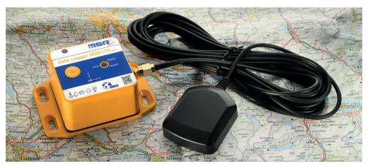
The tamper-proof MSR175plus GPS data logger captures potentially damaging shock events as well as recording the geographical position of the event. This robust data logger ensures compliance with transport specifications and provides indispensable data for identifying liability in the event of damage as well as helping with insurance claims.
